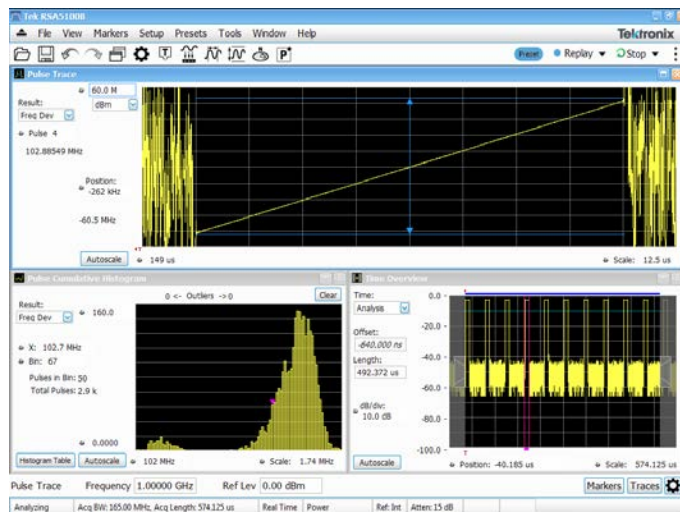
FIGURE 21. Frequency Deviation of a linearly chirped pulse.
